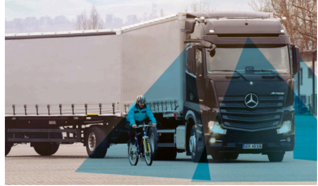
It can support the driver in entering and exiting intersections, backing up and maneuvering, and increase safety.
