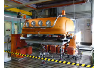
Hydropulse test stand for simulating pot holes and rough road conditions.
